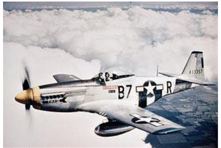
P-51 44-13357 of 374th Fighter Squadron, an early D-model, without the fin strake; 75 US gallons (62.5 imp gal; 284 L) drop tanks are on the wing racks.
